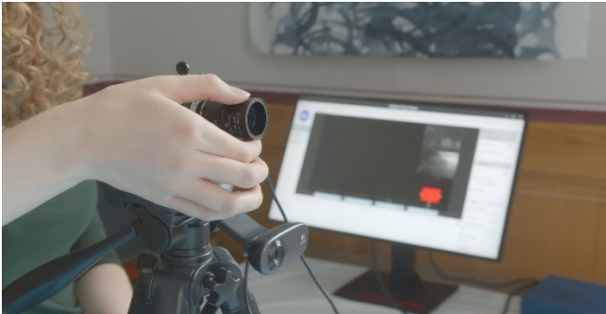
Left: Visual information about the brushstroke's trajectory and velocity is captured by a Dynamic Vision Sensor (DVS) camera. It encodes changes of light intensity with ultra-low latency. Photo by Marcus Nebe, © VG Bild Kunst / Liat Grayver.
