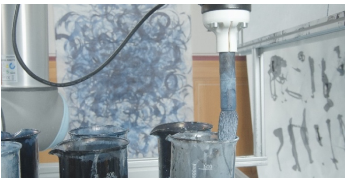
Left: Six glass containers are installed as a palette for the painting robot. In order to be able to create gradients in the painting process, the containers are positioned in the following order: blue or black ink, water, water, white ink, water, water. Photo by Marcus Nebe, © VG Bild Kunst / Liat Grayver.
